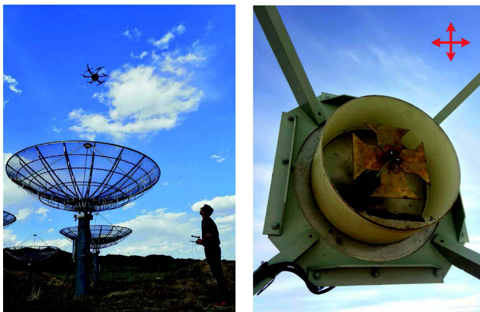
Fig. 2. (Color online) A dish antenna (left) and feed antenna (right) in the TDPA.
