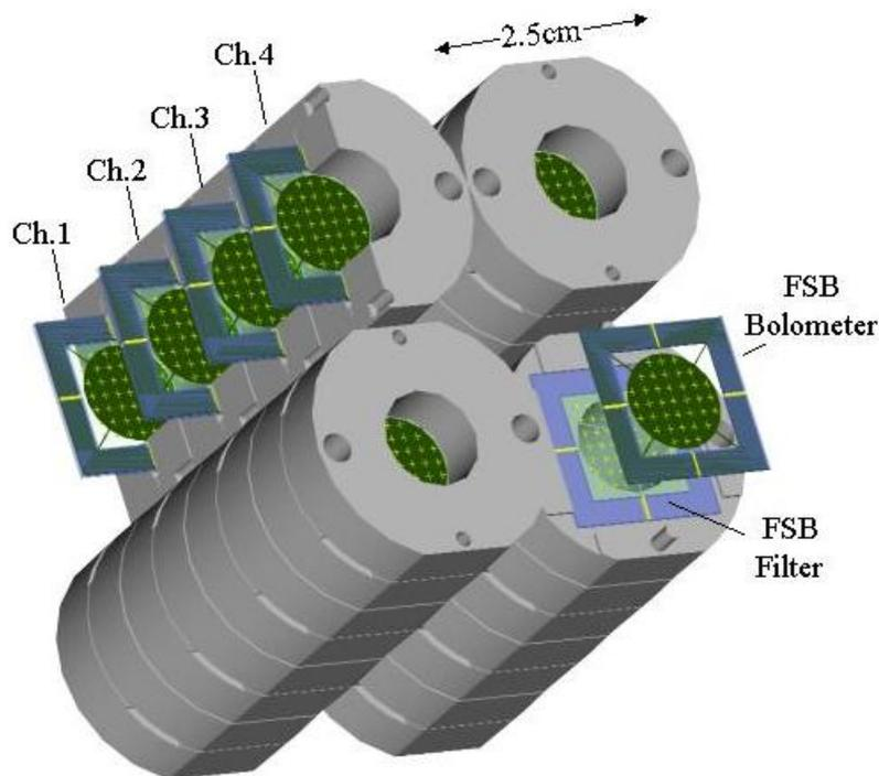
**Figure 2.** An exploded cartoon view of a possible four pixel photometer configuration for SPEED. The final photometer configuration will depend on some parameters of device processing which are being explored at the time of this writing. Notch filters and low-pass filters are not shown. Four FSB channels absorb in atmospheric windows at 2mm, 1.5mm (two channels), and 0.85mm.
