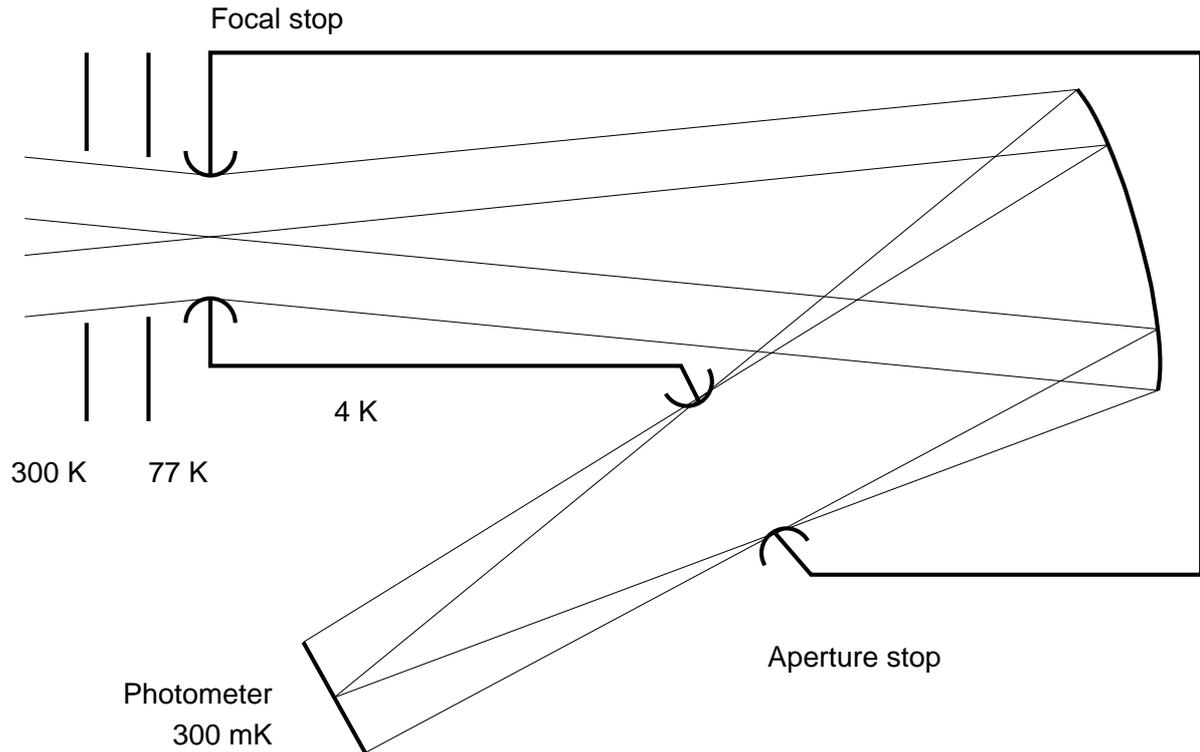
Figure 4. A conceptual view of the optical layout of the SPEED radiometer.
