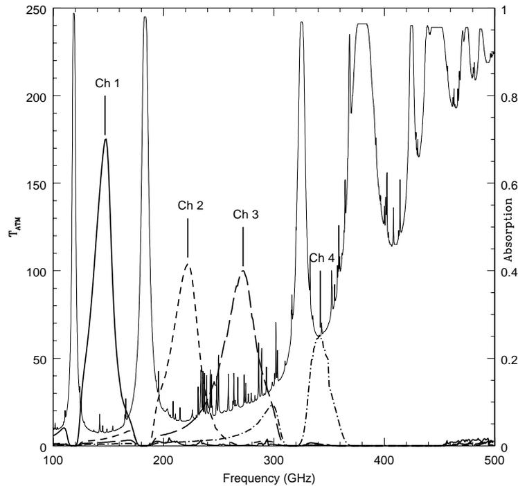
**Figure 1.** Model of the effective atmospheric temperature with 2 mm of precipital water vapor at the LMT site. Overlaid on the model are the predicted SPEED passbands.
