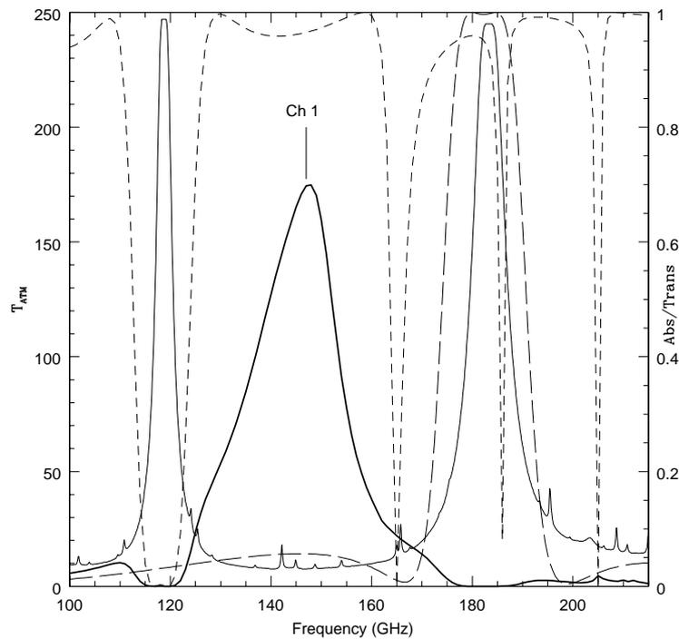
**Figure 3.** SPEED channel overlaid with a model of the atmosphere with 2 mm of precipitable water vapor. The transmission response of the two adjacent notch filters is shown with dashed lines. The sharp dips in transmission of the notch filters is an artifact of the HFSS model.
