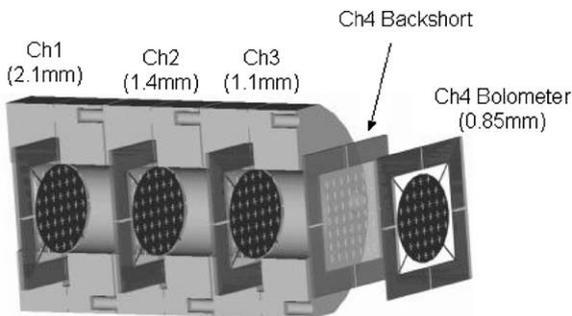
Fig. 1. Schematic of the SPEED detector array assembly for one spatial pixel.
