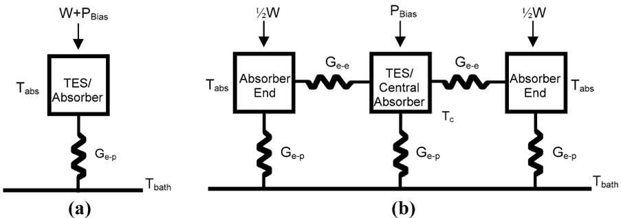
**Fig. 2** (a) Thermal model for an ideal THM.  $W$  is power incident on the absorber,  $P_{Bias}$  is Joule power due to the voltage bias of the TES,  $T_c$  is the operating temperature for the TES, and  $T_{bath}$  is the cold stage temperature. (b) Thermal model for a thermally disconnected THM. The ends of the absorber are at temperature  $T_{abs}$ , while the TES and the central portion of the absorber nearby the TES are at  $T_c$
