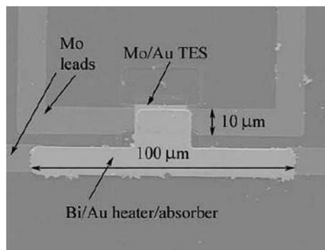
THM is weak. In an optimized THM the electrons in the absorber and TES are in thermal equilibrium and the hot-electron effect provides the thermal isolation for the bolometer. (i.e.  $G_{e-e} > G_{e-p}$ ). The measurements of the thermal properties of the test device presented here will be used to optimize the design of future THMs.
