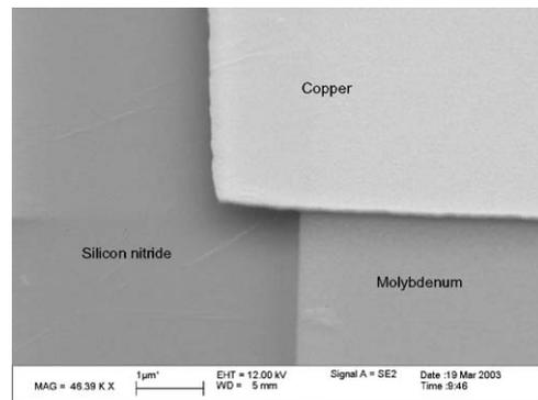
Fig. 2. SEM of the Mo/Cu edge of a test TES. Plasma etching undercuts the Mo layer by  $\sim 300 \text{ nm}$ , and produces a Cu overhang which eliminates superconducting shorts along the sides of the device.
