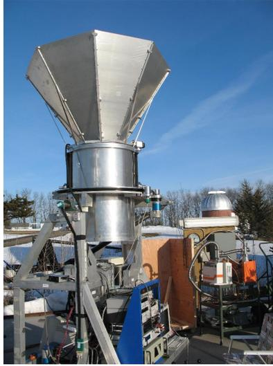
Figure 5. The MBI instrument observing the zenith at Pine Bluff Observatory in the winter of 2008. The octagonal structure above the cryostat is a ground shield.
