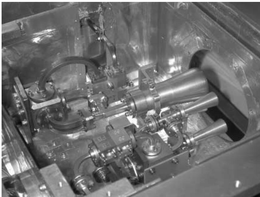
FIG. 6.—View inside the Dewar. The *W*-band polarimeter horn (top, small horn) is aligned with the optical axis of the telescope, and the two *W*-band horns underneath are for the *W*-band anisotropy radiometer. The *Q*-band polarimeter horn is tilted 4° toward the *W*-band polarimeter horn due to the curvature of the focal plane when off of the optical axis. [See the electronic edition of the Supplement for a color version of this figure.]
