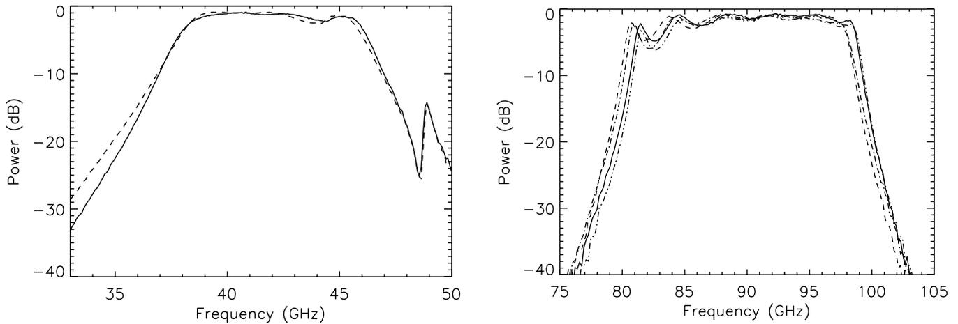
FIG. 3.—*Q*-band (left) and *W*-band (right) filter bands. The data show transmission (normalized to input signal) through the filters. The different lines denote each of the filters used in the radiometers.
