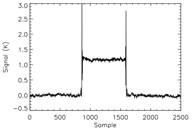
FIG. 9.—Example of automatic calibration sequence in  $Q$ -band (left) and  $W$ -band (right), 25 Hz data rate. Placing the dielectric film at a  $45^\circ$  angle in front of the radiometers creates a relatively small polarization signal that is easily detected.
