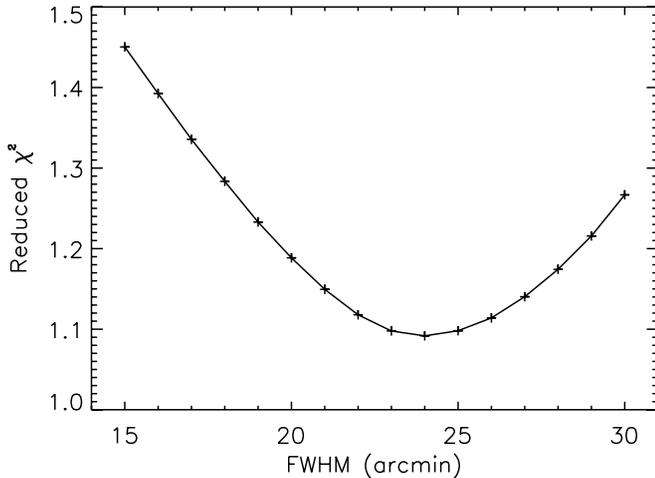
FIG. 8.—Determination of the  $Q$ -band beam size. A least-squares fit between observations of Tau A and a point source convolved with a Gaussian beam was used to determine the beam size. The measured FWHM beam size of the  $Q$ -band polarimeter is  $24' \pm 3'$ . The number of degrees of freedom is 347, corresponding to 347 HEALPix pixels ( $3.4'$  resolution,  $n_{\text{side}} = 1024$ ) that cover a  $1.1 \text{ deg}^2$  circular sky area centered on Tau A.
