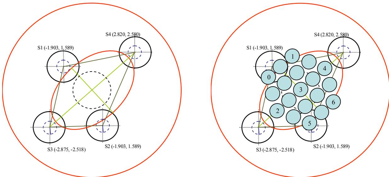
Fig. 2. Schematic diagram showing the optical layout of the MBI beam combining telescope. The left image shows the position of the 4 illuminating corrugated horn antennas with respect to the primary and secondary mirrors. The right image indicates the position of the detector array of 19 spider-web bolometers (the numbers are referred to later).
