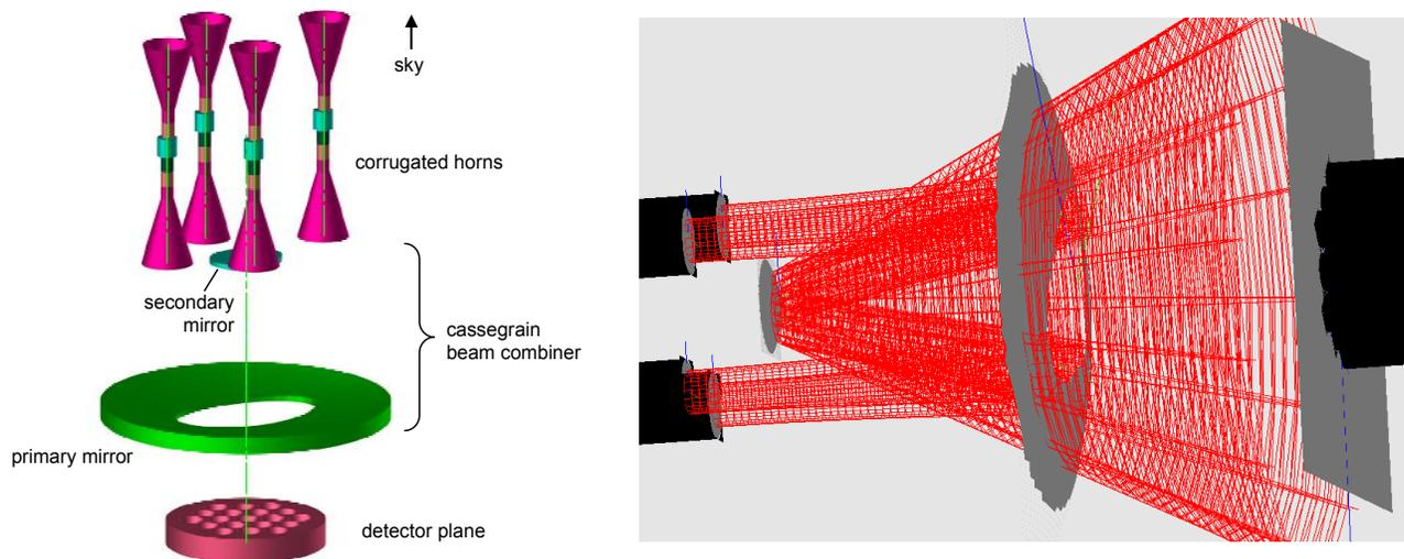
Fig. 1. An artists impression of the Millimeter-Wave Bolometric Interferometer (left) and the telescope as modeled in MODAL (right). The back-to-back feed system that illuminates the primary mirror can be clearly seen, as can the detector plane consisting of 19 spider-web bolometers. Because of the positioning of the of the horn antennas the aperture in the primary can be seen to be elliptical, however truncation at the primary still occurs.
