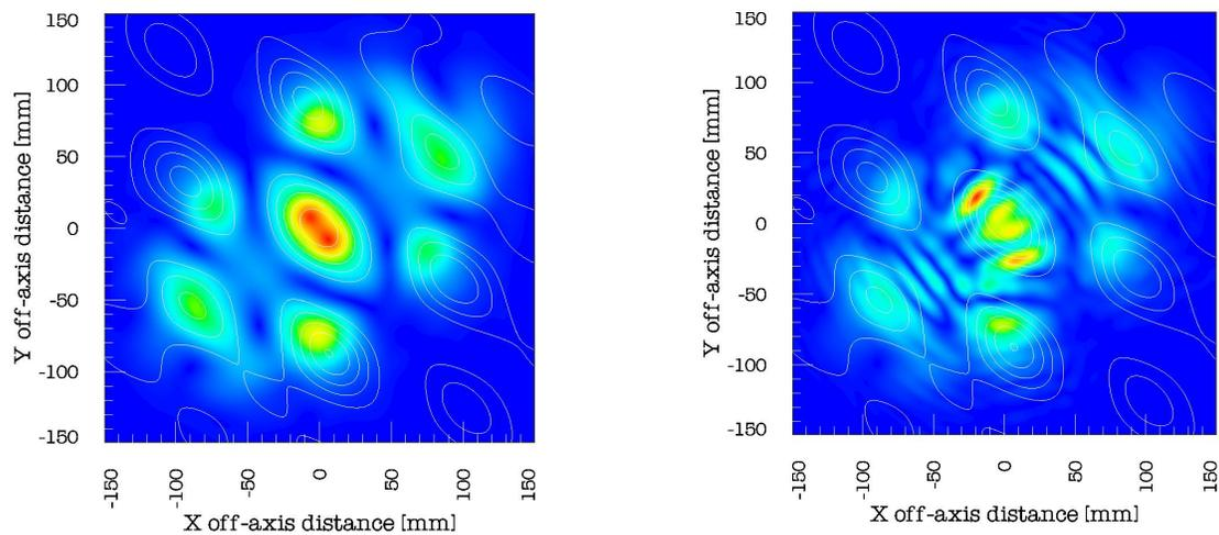
Fig. 6. The field at the image plane with the color map representing a Gaussian beam mode analysis and the contours a physical optics analysis (left). A Gaussian beam mode analysis with the field that passes through the aperture on reflection at the primary taken into account (right).
