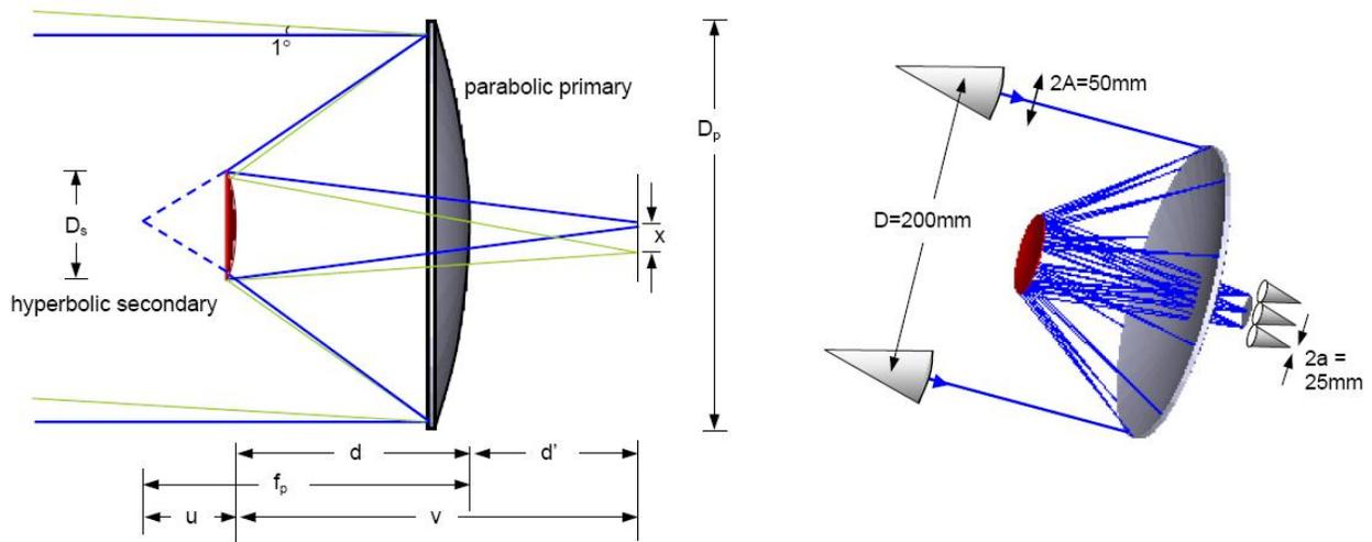
Fig. 3. Schematic diagram of the MBI optical system where  $D_p$  is the diameter of the primary mirror,  $D_s$  is the diameter of the secondary mirror,  $d$  is the distance between the mirrors,  $d'$  is the distance from the primary to the image plane,  $f_p$  is the primary focal length,  $f_s$  is the secondary focal length,  $x$  is the fringe separation,  $D$  is the baseline,  $A$  is the radius of the feed horn and  $a$  is the radius of the detector horn [8].
