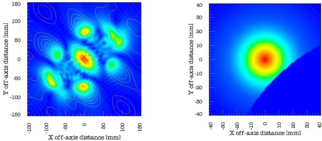
Fig. 5. The field at the image plane of the telescope (left) where the contours show the intensity with no truncation at the primary aperture and the color map takes into account this truncation. The truncated beam from a single source on reflection at the primary mirror (right).
