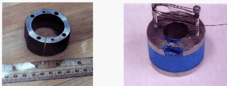
FIGURE 6. Miniature split-coil superconducting magnet for heat switch. The bore diameter is 1.5 cm. (Left) : Side magnet shield. In order to reduce eddy current heating in the magnet, a slot has been machined in the shield. (Right) : Coil.
